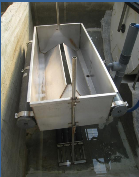
The SAFF-13 floating foam fractionator at the Syrian Asmak Company, Tartous Syria installed in a marine RAS producing Gilthead sea bream ( Sparus aurata ).
