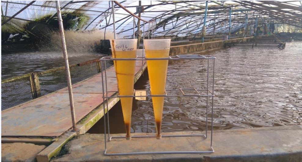
Imhoff Cones used to measure the volume of biofloc in the water column at Chambo Fisheries four times daily.
