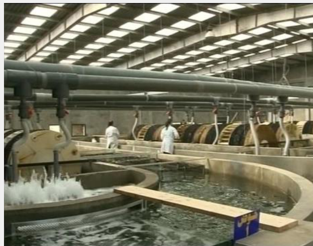
RAS technology tailored for several marine linefish species where water velocities are tuned to achieve 25-35cm/sec favouring rapid growth and improved meat texture as well as reduced Feed Conversion Ratio's (FCR).
