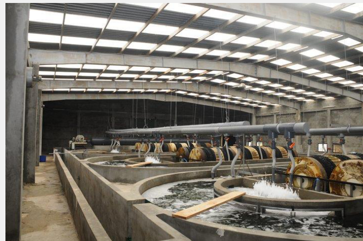
RAS technology tailored for several marine linefish species where water velocities are tuned to achieve 25-35cm/sec favouring rapid growth and improved meat texture as well as reduced Feed Conversion Ratio's (FCR).
